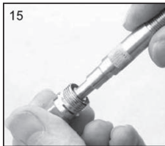
15. Fit Seal to Housing (10).
