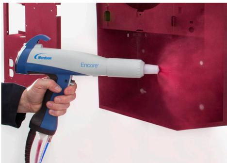
Encore HD Manual Gun spraying dry-blended metallic powder.
