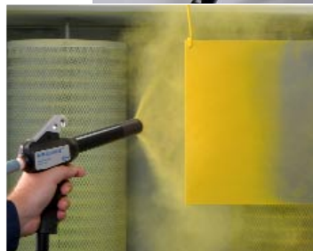
Nordson AeroCharge manual spray gun and control unit; (inset) Close-up 'point and shoot' accuracy delivers unprecedented coating capability with uncompromising finish quality.
