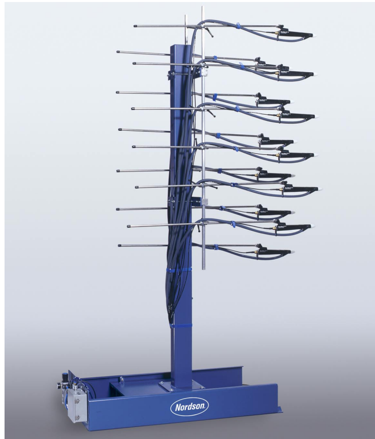
Nordson horizontal gun mover shown here with fixed gun stand
