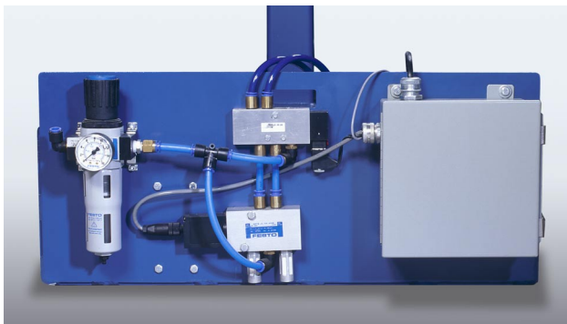
The servo-pneumatic valve eliminates wobble at the point of spray for more precise spray application.
